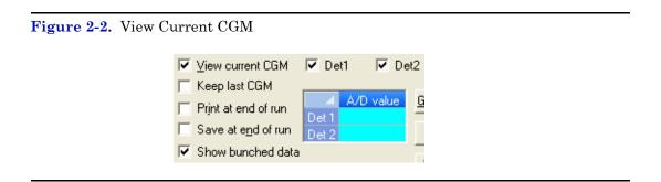
The chromatogram displays in the chromatogram window. If the chromatogram contains one trace, the *Det1* checkbox is automatically checked; if the chromatogram contains two traces, the *Det1* and *Det2* checkboxes are automatically checked. To remove a trace, uncheck its detector checkbox.
